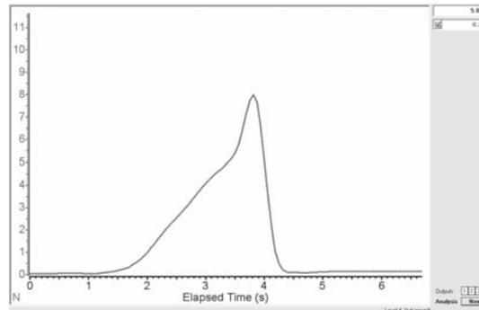
The graph shows a small paper tube being crushed until it collapsed.
