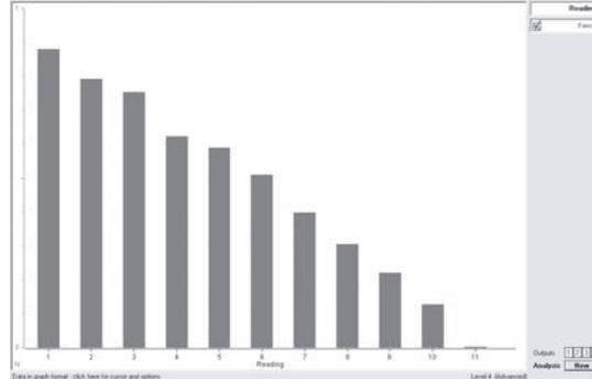
The graph shows how the force is reduced as a 100 gram mass is moved along the metal plate by 1 cm at a time.
