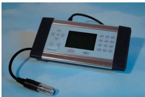
1. Connect the Sound Wave sensor to channel 1 of DataVision.
