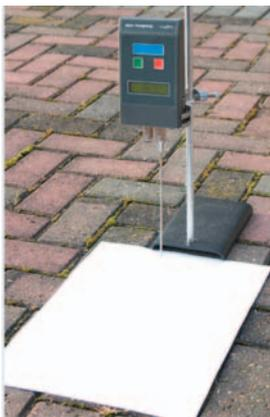
1. Find a secure and weather protected place for the datalogger. Avoid direct wind which could affect the result.
