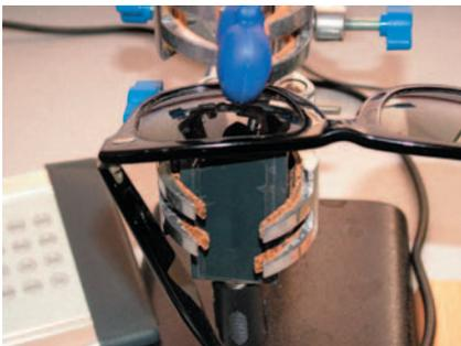
1. Connect the UV sensor to a channel of the LogIT Datalogger.
