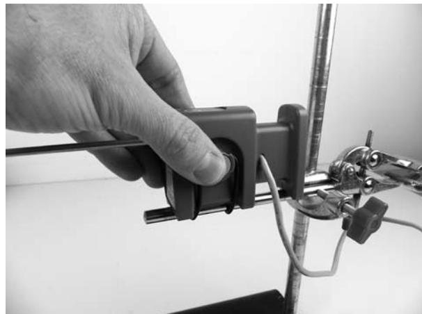
2. Place the fan close to the probe and place a small folded piece of paper towel (about 1 x 4cm) on the tip as shown.
